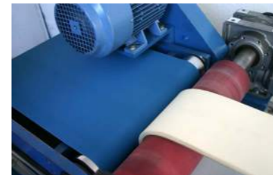
Special coating materials available possible ie. Linatex, -Correx, Cell Rubber, Natural Rubber or soft PU
