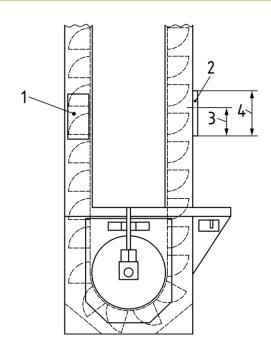
Bucket spacing < 280 mm; Required vent height ≥ 1,5 x bucket spacing;
